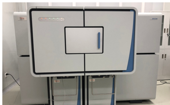
High resolution isotope ratio mass spectrometer (253 Ultra)
