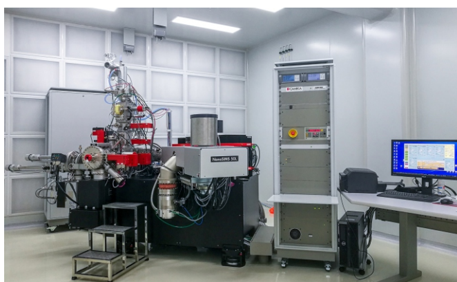
Nano-scale secondary ion mass spectrometer (NanoSIMS)
