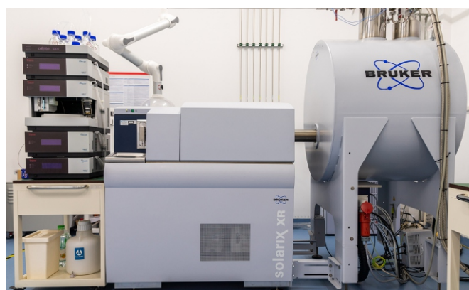
Fourier transform ion cyclotron resonance mass spectrometer (FT-ICR MS)
